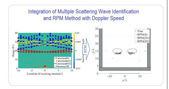
Moreover, this technology succeeded to improve the accuracy of detection by discriminating between human body and other objects. Since the surface of human body is always shaking, this technology catches the information of such shaking and utilizes it as a signal to process for human specific imaging. On the other hand, the motion speed of each part on shaking human body is about 0.1 m / s called as micro Doppler and it is necessary to estimate the Doppler speed on high-resolution capability.
