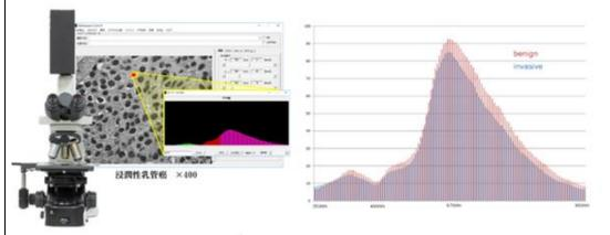
The Hokkaido satellite's hyperspectral camera is installed in the microscope. Obtain spectral data
